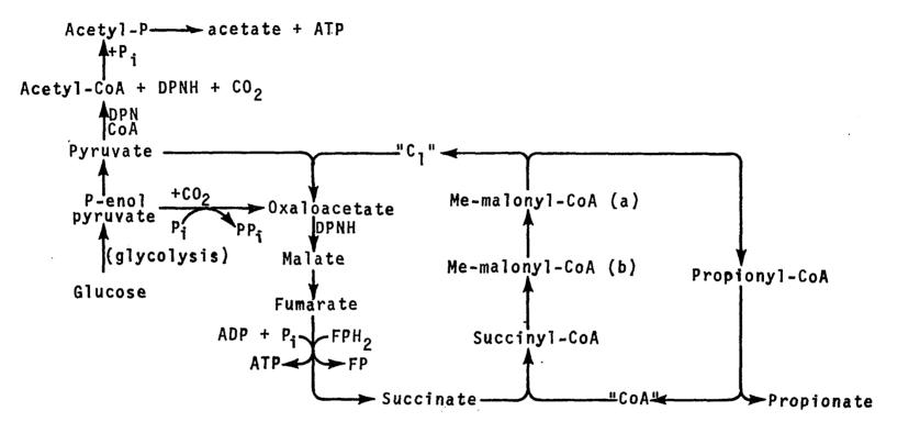
Fig. 1. Reactions of the propionic-acid fermentation and the formation of acetate, propionate, carbon dioxide, and ATP
